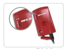
LED On: On Charging □ LED Off: Fully Charged
