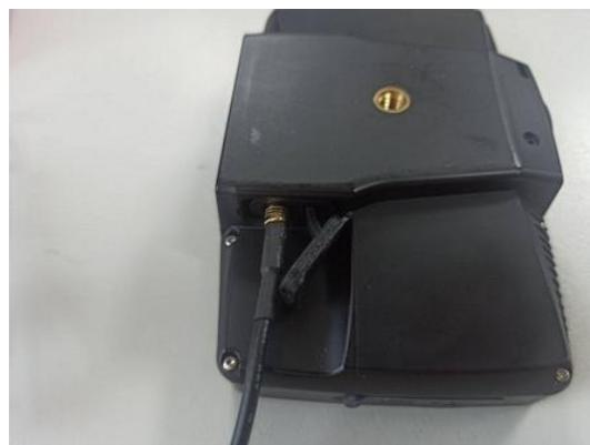
3. When unplugging the external antenna, hold the connector and unplug it vertically.
