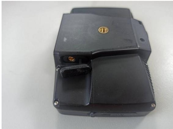
2. Plug in the GPS antenna connector vertically into antenna jack.
