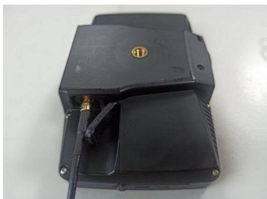
**4.** Push down the top of rubber cover into antenna jack first. Then push down the bottom of rubber cover to close it.
