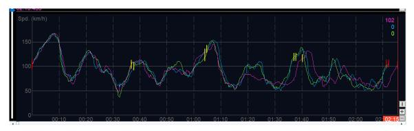
In Trace Map View, using the color tags on the trace or on the graph table to mark the position for define accelerate point or break point purpose.
