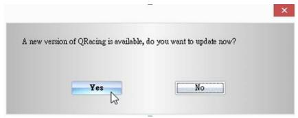
For LT-Q6000, LT-6000S, LT-6000S2, LT-8000GT models: POWER OFF the device and connect to your PC with internet. QRacing will auto detect and update to the latest device firmware and Trackmap version. You can also update the latest version of firmware and Trackmap by click QRacing software [Update] --> [Update device firmware] [Update device tracks].
