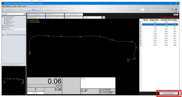
You can set the coordinate position for the beacon setting. Go to QRacing Menu --> [Beacon] --> [Input Reference Coordinate]. Input the Latitude and Longitude to mark the position of the beacons.
