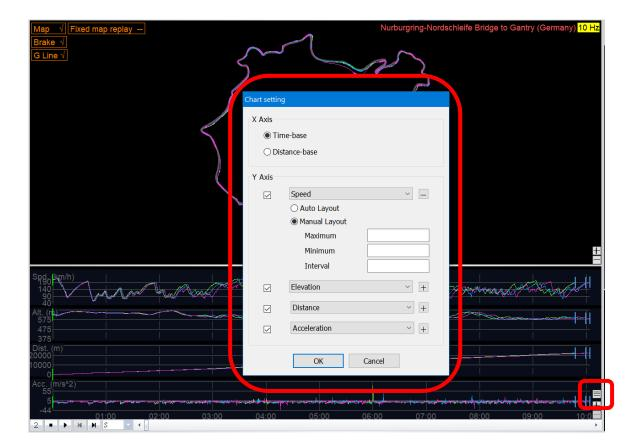
**8.5.2.8** Window resizing: If you want to resize the window horizontally/vertically, point to any edge of the window. The mouse pointer will change to indicate that you can resize the window. Grab the edges and drag the window to the new size.
