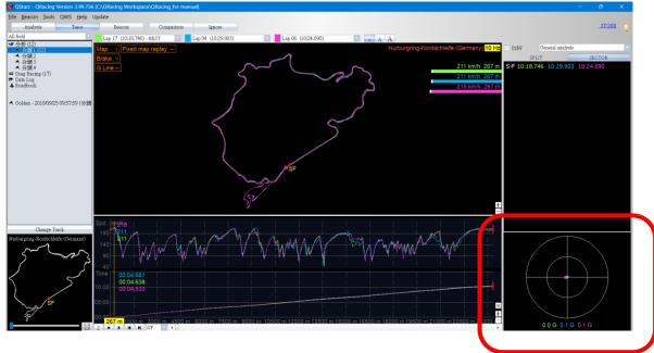
8.5.2.3 Accel line (acceleration) / Braking line (Deceleration): It shows the accelerate and decelerate lines on the trace. You can compare the accel line and braking line for difference laps. (The thick line presents the braking zone, and the thinner lines present the acceleration zone.)
