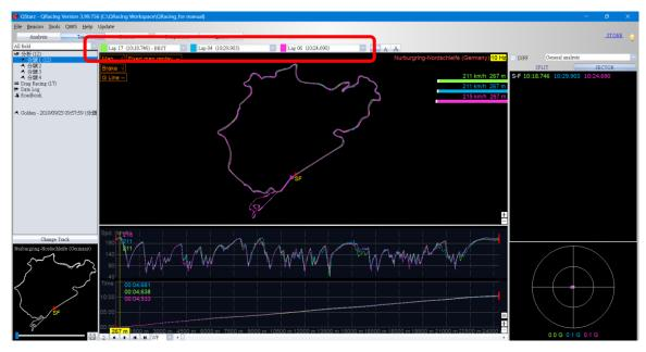
When using **Time-base**, the speed difference line will be shown on the graph by two laps comparison.
